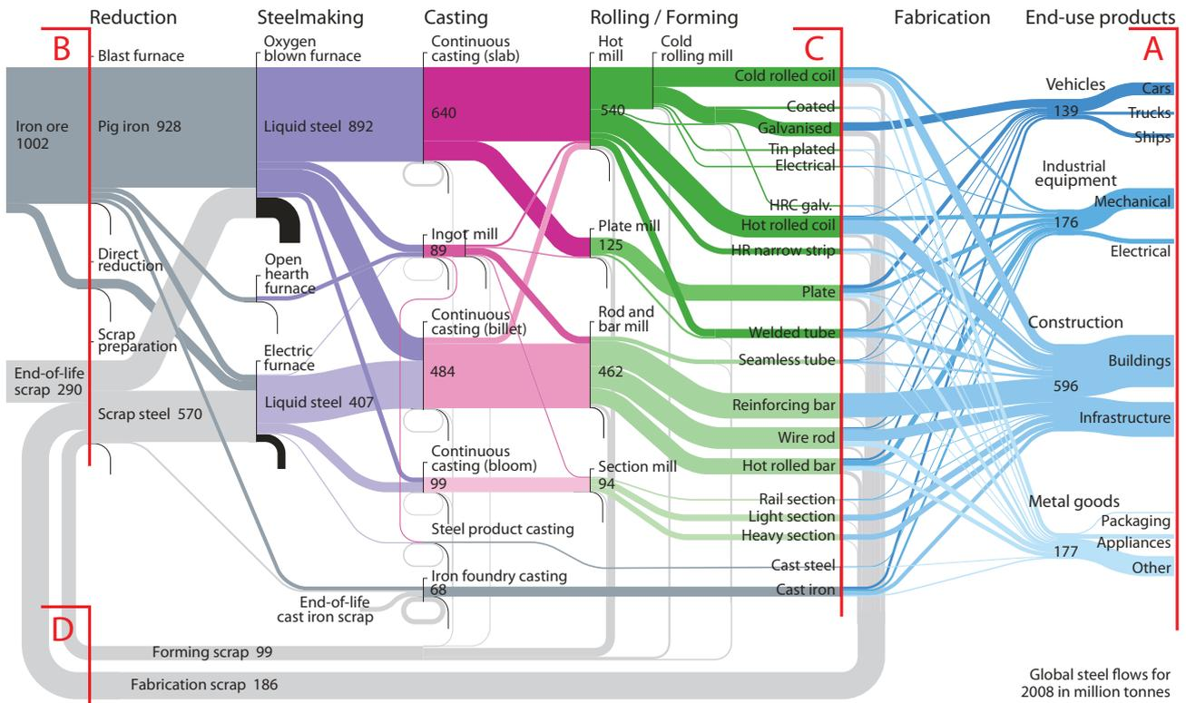
Steel is the world's most used metal, by far, and we make over 200 kg of liquid steel each year for every person alive. The figure above illustrates the 'flow' of steel through the world economy in 2008, with the width of each line proportional to the mass of steel produced. Since 2008, the volume of steel production has increased, but the proportions of the flows have remained similar.
