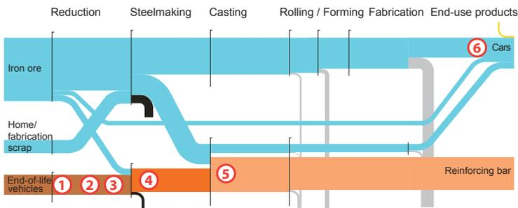
1. Steel-bearing products at end-of-life could be disassembled with more care, to maintain larger components and avoid alloy mixing. In some construction projects, I-beams could be re-used directly creating the same business opportunity exploited by authorised own-brand used car dealers.
