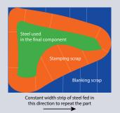
Half of all sheet steel is scrapped during manufacturing: in this example, the car panel doesn't tessellate, and extra material is needed for grip while it is shaped
