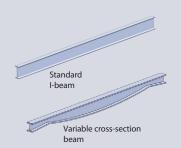
Floors deflect most furthest from the walls, so floor beams should have a variable cross-section. Standard I-beams use 30% more steel than necessary, to no benefit
