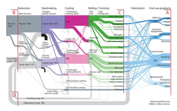
Steel is the world's most used metal, by far, and we make over 200 kg of liquid steel each year for every person alive. The figure above illustrates the 'flow' of steel through the world economy in 2008, with the width of each line proportional to the mass of steel produced. Since 2008, the volume of steel production has increased, but the proportions of the flows have remained similar.
