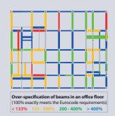
Steel framed commercial buildings must meet the safety standards of the Eurocodes, but on average are currently over-specified by a factor of two
